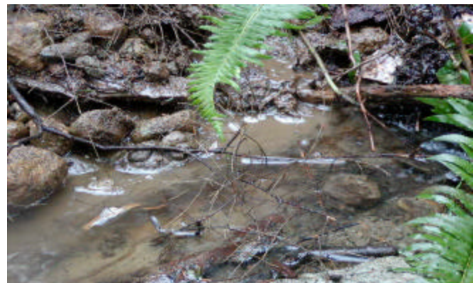
During same storm, creek discharge 0.2 l/s with turbidity of 1000 ntu. Immediate effect on stream (discharge 400 l/s with turbidity of 10 ntu) was to increase the turbidity by 1 ntu.
